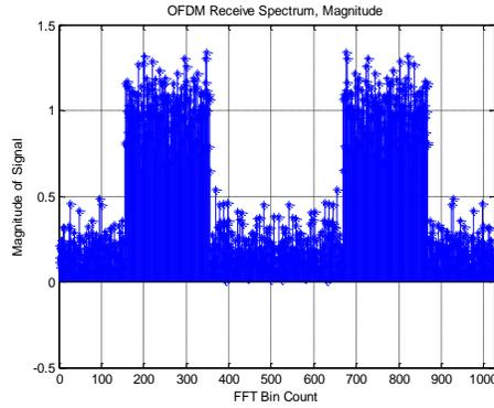
**Figure 8:** shows a OFDM received signal spectrum. It shows the magnitude of signal received with respect to the FFT bin count for the signal received at Receiver.
