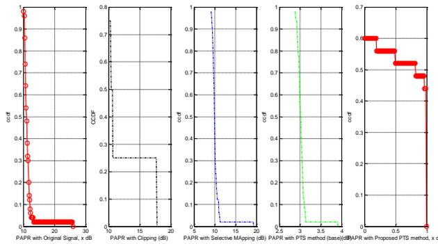
**Figure 12:** Depicts the Comparative view of PAPR values with respect to CCDF for all the techniques used for the simulation. It is clear from the figure that line shown in red for the proposed having lower values of PAPR for all values of CCDF.
