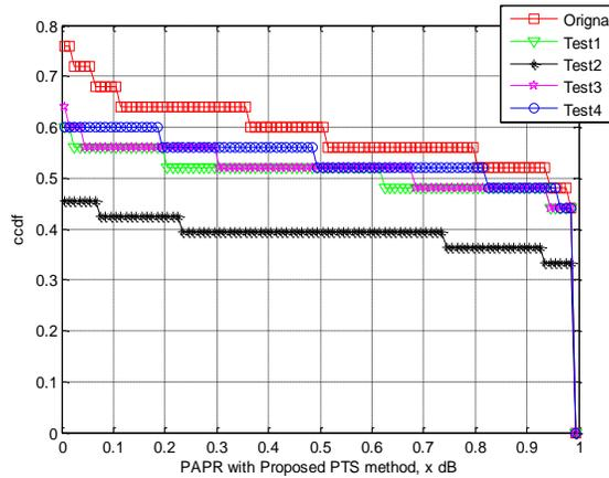
**Figure 13:** shows a comparative view of obtained PAPR values with proposed system by taking various number of sub-blocks for experiment purpose. It is clear from the figure that we are getting minimum PAPR values while taking 4 sub-blocks in proposed work.
