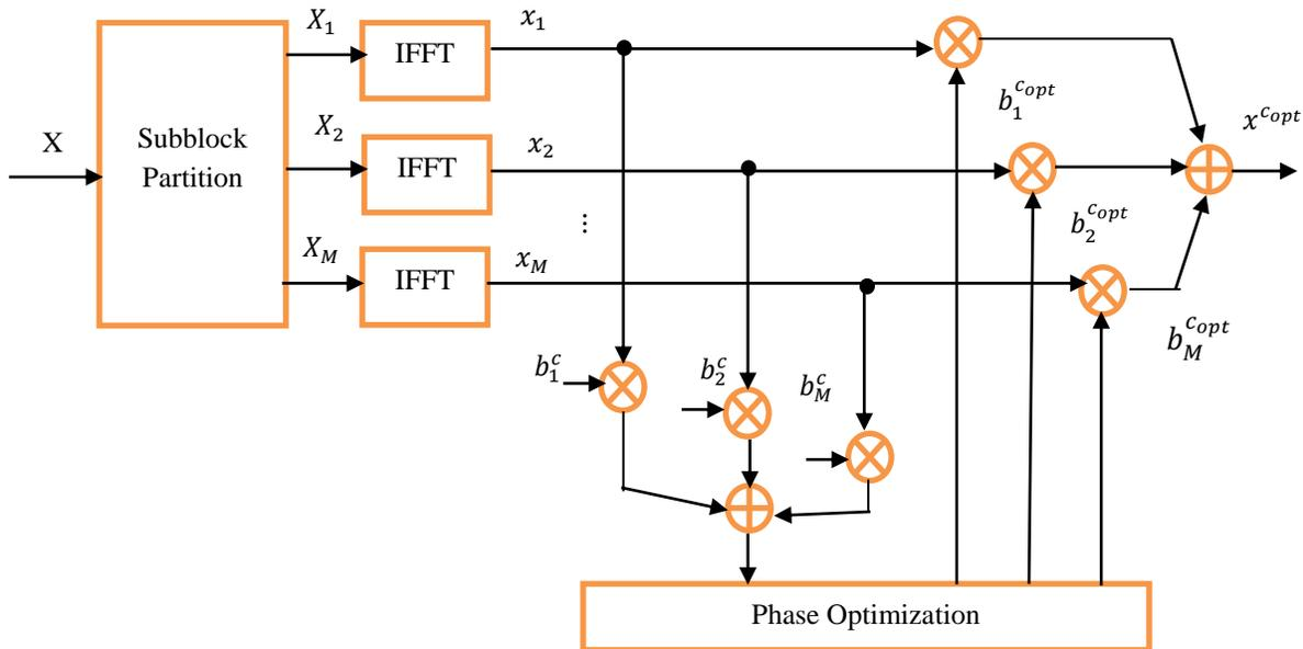
**Figure 1** Block diagram of the conventional PTS scheme
