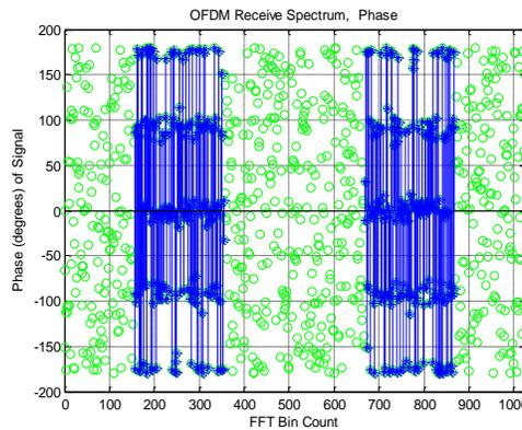
**Figure 9:** shows phase information of received signal spectrum. In figure, phase of the received signal is plotted with respect the FFT bin count for the signal received at the receiver after adding noise within the channel.
