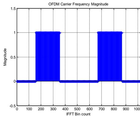
**Figure 4:** Shows the Magnitude of signal with respect to IFFT bin count for transmitted OFDM signal.
