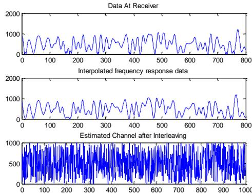
Figure 11: shows the comparative view of signal magnitude for data received at the receiver, interpolated frequency response data and estimated channel after interleaving for the proposed work.
