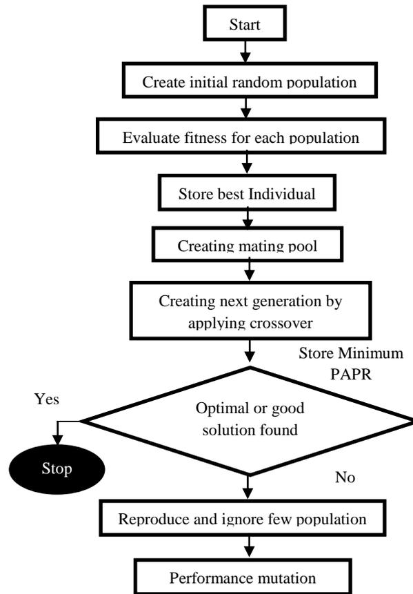
**Figure 4:**Flow chart of Genetic Algorithm Optimization.
