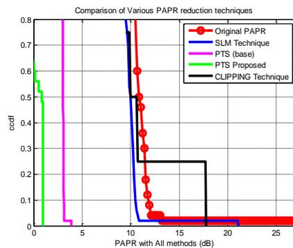
**Figure 17:** shows a comparative view of PAPR with respect to different values of CCDF for all 4 techniques used for the simulation while decreasing value of SNR or increasing effect of white Gaussian noise in channel side model (Signal to Noise ratio = 5). From figure, it is clear that the proposed PAPR reduction technique perform much better than other techniques and also outperform the PTS technique proposed in [28].
