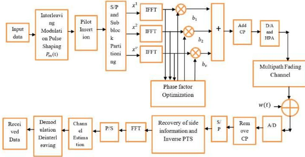
Figure 3: Block diagram of OFDM system using proposed PTS combined with sequence interleaving and phase shifting.
