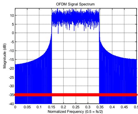
Figure 7: shows a signal spectrum of Proposed OFDM system. X axes shows the normalized frequency defined for proposed system and Magnitude in dB is shown in Y axes for transmitted OFDM signal.
