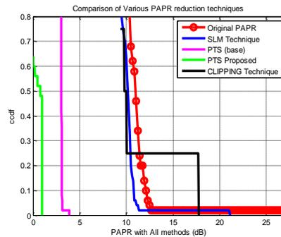
**Figure 16:** shows a comparative view of PAPR with respect to different values of CCDF for all 4 techniques used for the simulation while increasing number of carriers in transmitter model (Number of carriers = 300). From figure, it is clear that the proposed PAPR reduction technique perform much better than other techniques and also outperform the PTS technique proposed in [28].
