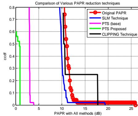
**Figure 14:** shows a comparative view of PAPR with respect to different values of CCDF for all 4 techniques used for the simulation. From figure, it is clear that the proposed PAPR reduction technique perform much better than other techniques and also outperform the PTS technique proposed in [28]. We are getting a very lower value of PAPR of approximately ~1 to ~2 dB by using the proposed optimized phase shifted interleaved partial transmit sequence method.
