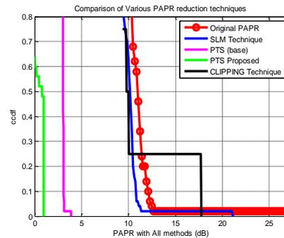
**Figure 16:** shows a comparative view of PAPR with respect to different values of CCDF for all 4 techniques used for the simulation while increasing number of carriers in transmitter model (Number of carriers = 300). From figure, it is clear that the proposed PAPR reduction technique perform much better than other techniques and also outperform the PTS technique proposed in [28].
